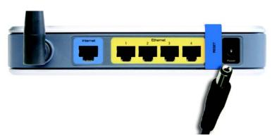
Figure 4-9: Connect the Power
